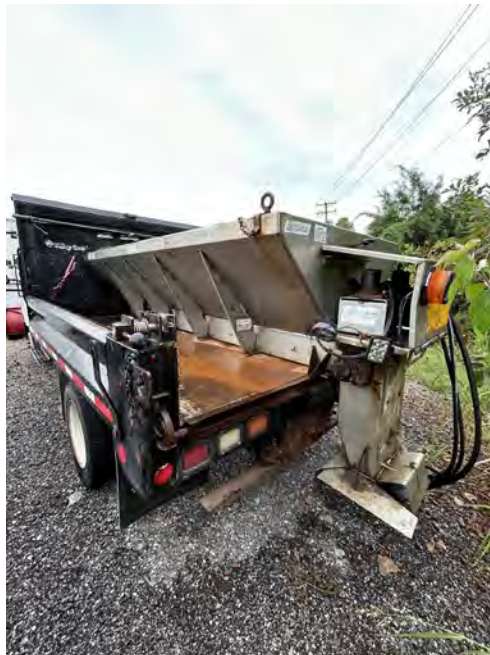
Henderson 4-cubic-yard drag-chain salt spreader and dump-body installation
